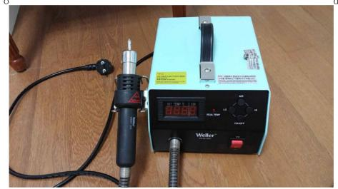
Use very good de soldering machine such as weller hot air gun (WHA 600 model) shown in the picture .
