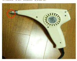
2. remove 3 crystal (25, 27 and 20 MHz) and resistor, capacitors etc as shown below. I recommend Weller hot air gut to take out components from the main board, it would take 4-5 minutes to be melterd.
