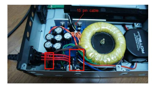
Mount Limear power module. Make sure the bottom of aluminium heatsink is well contact with botom chassi ( for proper cooling of heatsink through bootom chassi ) and screw 4 bolts ( except the center boalt) .
