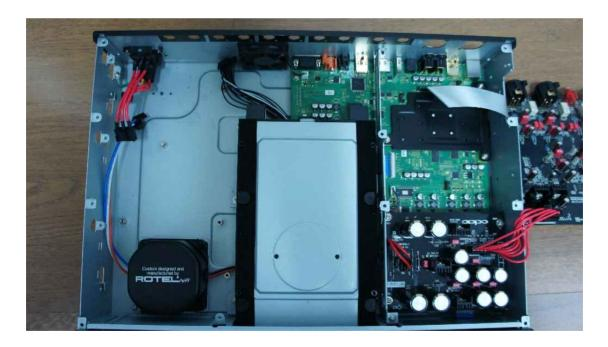
Take out metal bracket which is located between powe module and BD rom driver and take out black plastik plate which is under the power PCB sticky ) .
