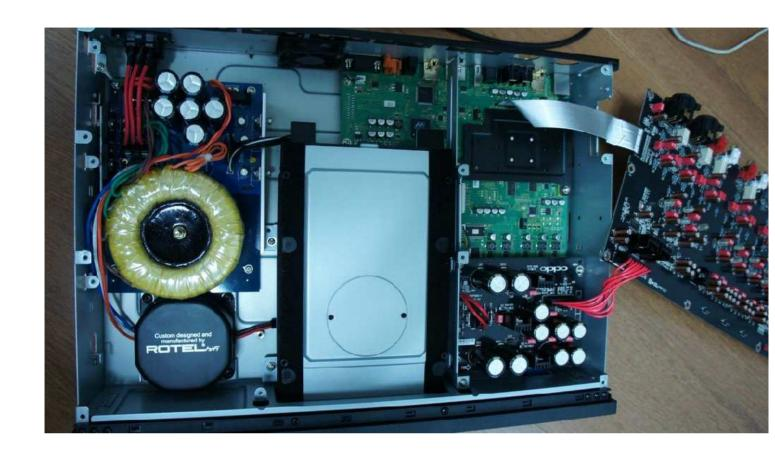
Replace the analog DAC board . Reassemble remaing parts .
