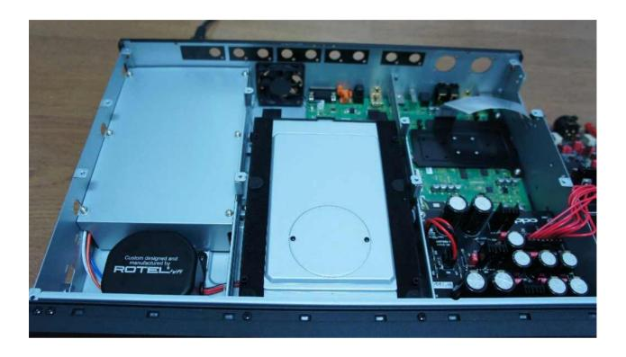
Open upper chassis and take out analog D/A board. You must unscrew many bolts. And take out metal box which covers power module.
