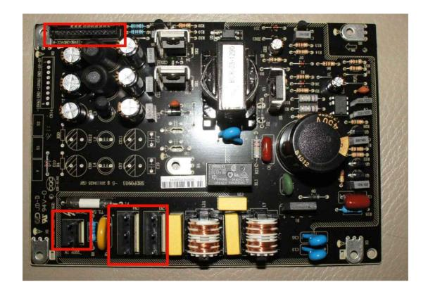
Take out power cord, two jumper cable and 15 pin cable. Unscrew 5 bolts
