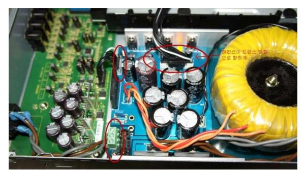
Connect power cord to wall outlet and check whether LED is on. (At this time, don't connect 15 and 6 wires jumper cables).
