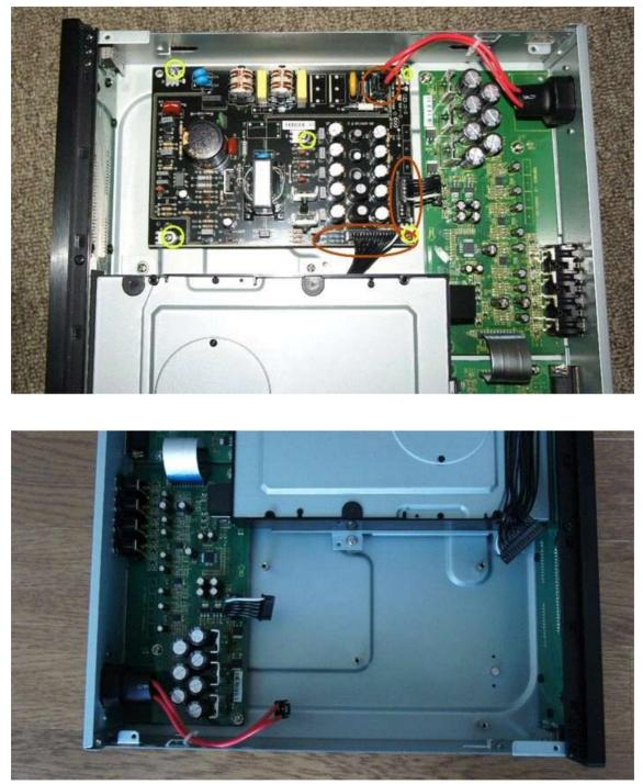
Unplug 1 power cord, 2 jumper wires and unscrew 5 bolts
