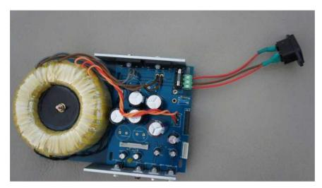
nsert 3 lead wires of power cable to green connector.2 red( or orange ) wires should be placed outer socket and 1 brown wire in center socket as shown in picture
