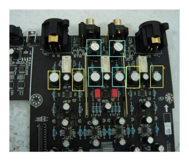
Coupling capacitors are a very important part where the sound signal passes directly. The function is to cut off DC voltage and pass only music signal, which is very directly related to sound quality.
